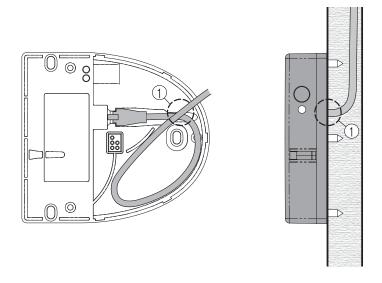
For unconcealed cabling, remove one of the outlets (circled in diagram below) in order to direct the cable neatly out of the GAT NET.Lock 7000 housing.
