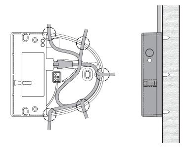
**NOTE!** Always leave sufficient reserve cable at the lock end (e.g., loop cable in the lock housing) for future service requirements.
