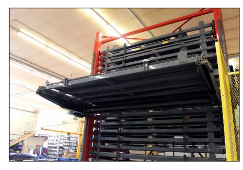
Vidir's VLS will store and retrieve material, utilizing available overhead space and deliver product to ground level for further processing and integration with production machines.
