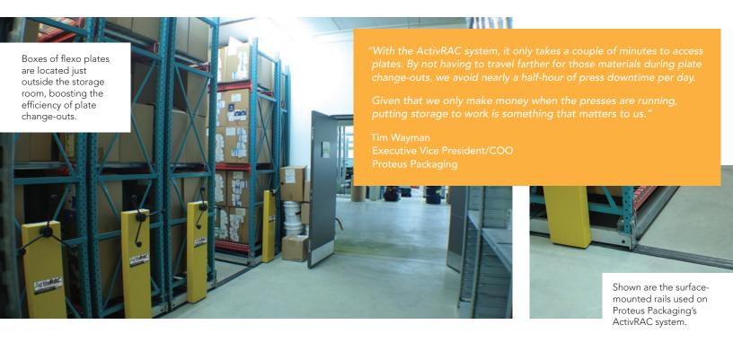
The mechanically-operated system at Proteus Packaging features five carriages matched to surface-mounted rails. Only one, three-foot aisle opens at a time to provide full access to needed materials. Remaining aisles stay closed. The ActivRAC system built for the package manufacturer is also 20 feet long and opens with minimal effort, thanks to an ergonomically designed handle and a mechanical-assist drive unit on each carriage.
