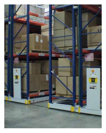
3. After carriages complete their movement the open aisle will be locked out and the control head indicator on either side of the open aisle will illuminate "Aisle in Use" - it's now safe to enter the aisle.
